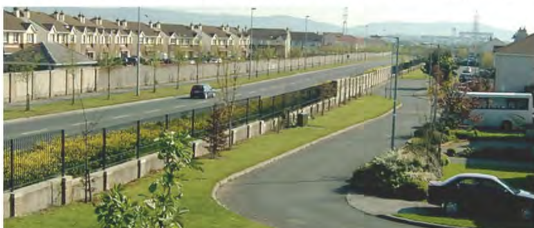
Figure 82 An example of inefficient design that restricts permeability (DMURS)
